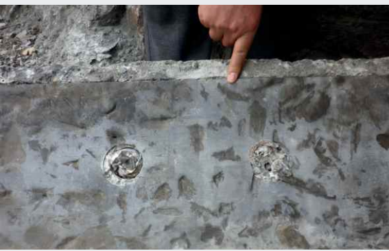
Excellent result: no damages on the Under Sleeper Pad
