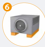
Bearing of building service equipment
