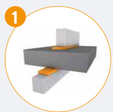
Decoupling of flanking transmission
