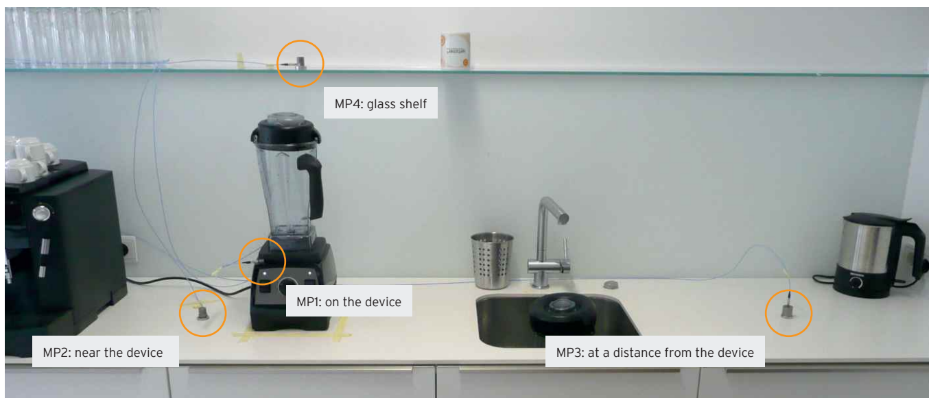
Experimental set-up: arrangement of the measurement points (MP) with acceleration sensors
