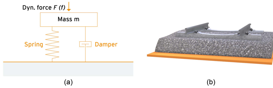
Fig. 5. Vibration isolation using under-ballast mats: (a) physical principle (single-mass oscillator); and (b) typical installation situation.
