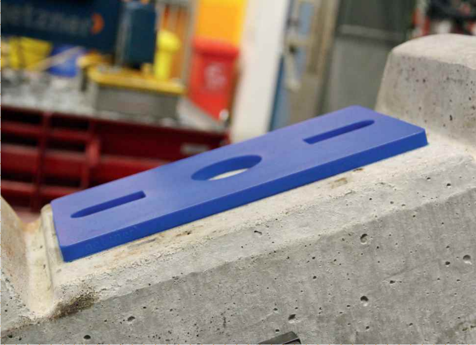
Getzner Sylodyn® baseplate pads add elasticity to the slab track.
