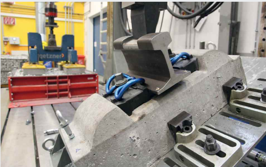
Baseplate pads are subject to intensive testing on the in-house test rig
