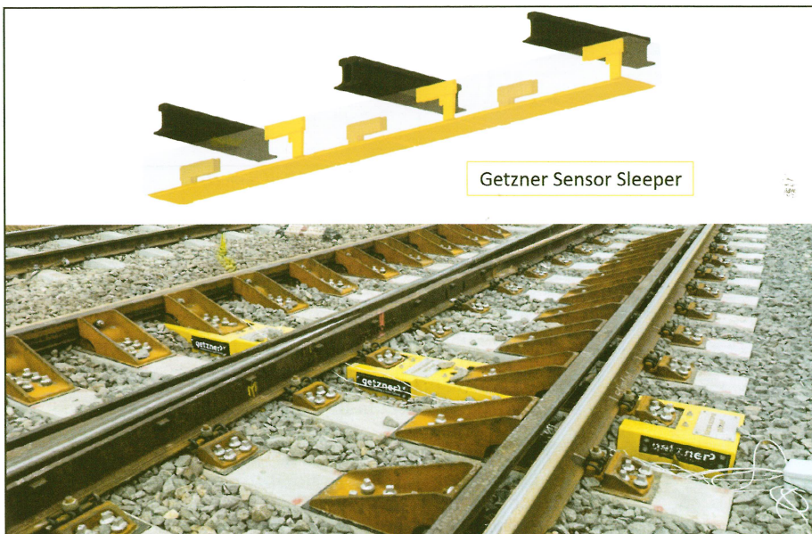
Fig. 14: Equipped demonstrator sleeper of the Shift2Rail project
