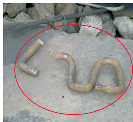
FIG. 8: Examples of typical problems encountered on heavy-haul railway lines throughout the world: destruction of ballast under concrete sleepers (left), fractured tensioning clamps (middle) and cracked sleepers (right) are mostly the result of excessively high dynamic loads
