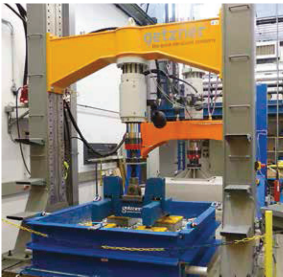
Simulation of high-axleload stress in the ballast box of the large test rig (left). Following the end of the test, the ballast grains remain embedded in the PUR material (right).
