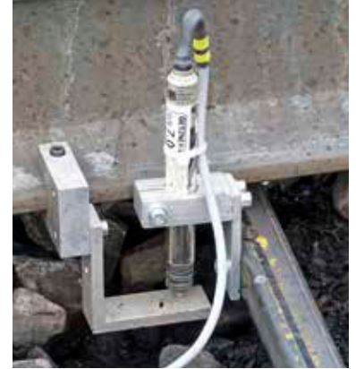
Fig 7. Deflection measurements at the transition under heavy haul conditions (top row). Determining the contact area in the lab (bottom row).
