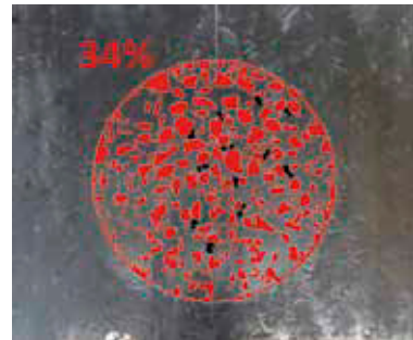
Fig 7. Deflection measurements at the transition under heavy haul conditions (top row). Determining the contact area in the lab (bottom row).
