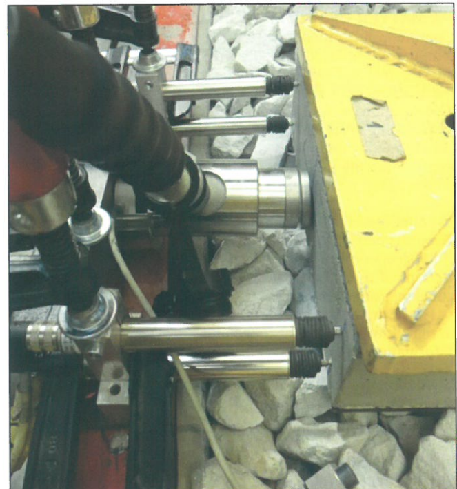
Fig. 3: Test set-up for the laboratory experiments, LTR measurement [3] (Photo: Sandro Gabl)
