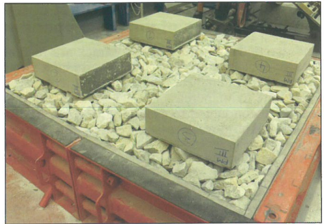
Fig. 2: Ballast box and arrangement of the test pieces for the laboratory experiments [3] (Photo: Sandro Gabl)
