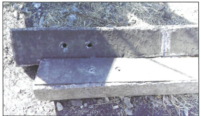
Fig. 15: Removed padded sleepers after more than 1 billion load tons of traffic – no signs of damage
